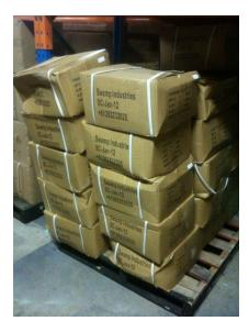
d) Tape All Edges to assist with carton condition during individual shipment
